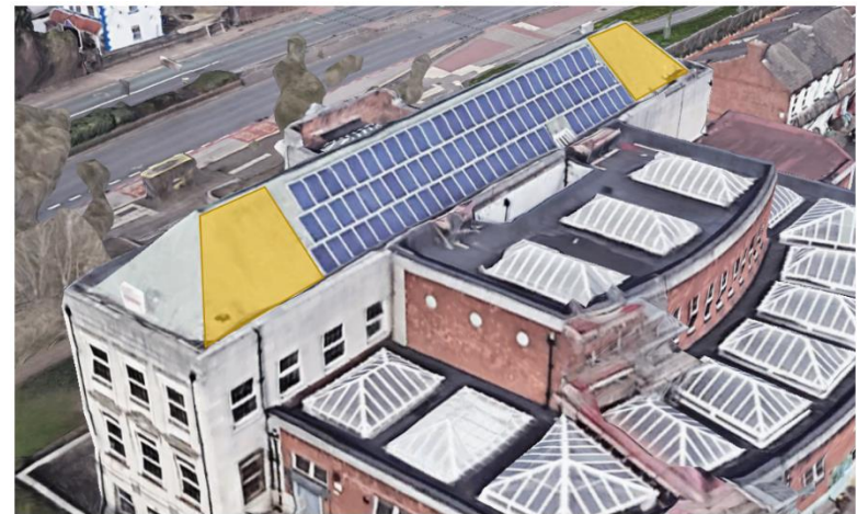
Existing PV system and rooftop areas suitable for solar PV highlighted, subject to structural survey.
